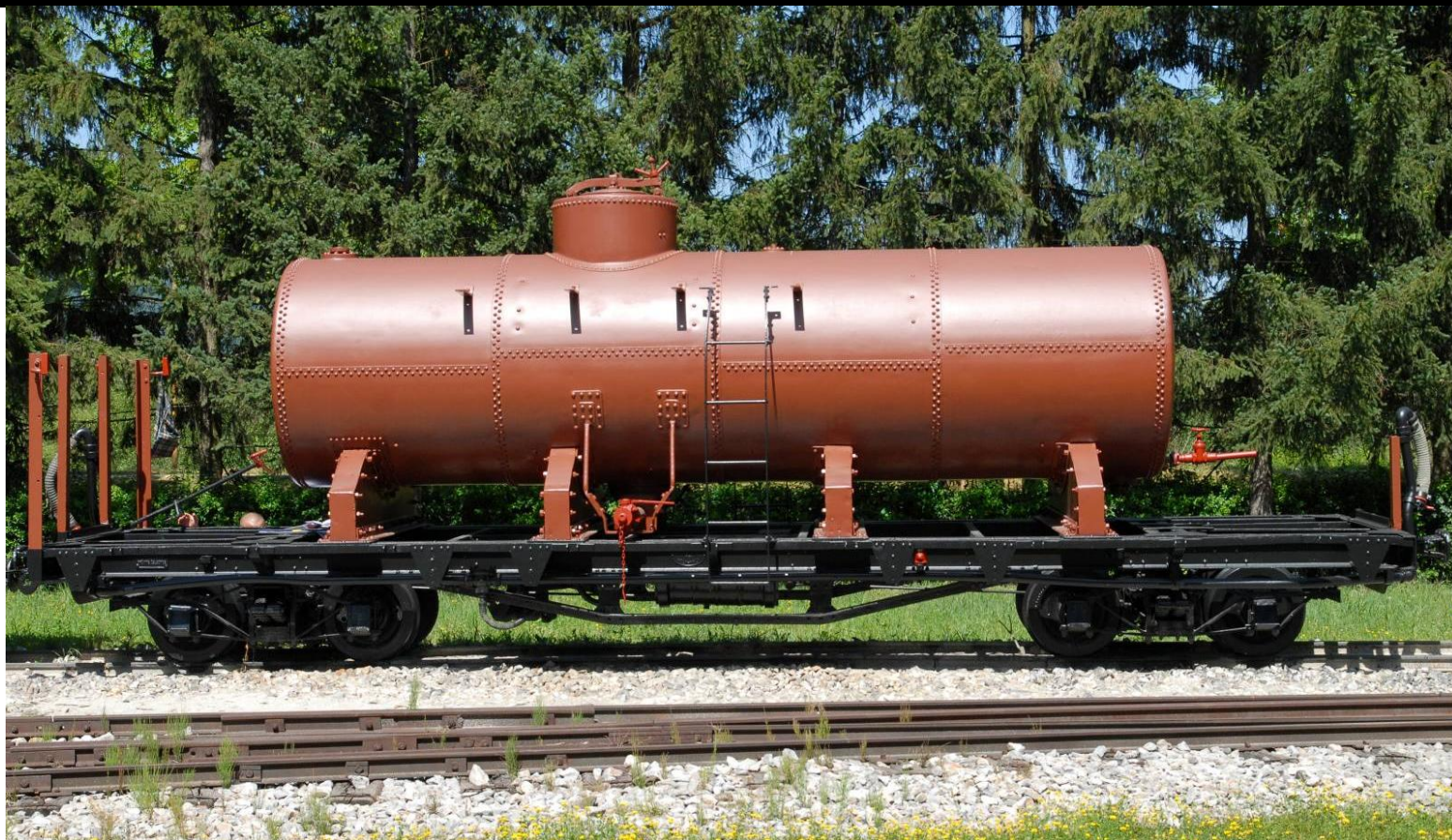
Four-axle tank wagon series R 84702 , operated on all narrow gauge lines, and, at the end on Paraćin – Zaječar railway line. This is a wagon with the MANUAL AIR BRAKE , with net weight 9470kg, carrying capacity 15 000kg, 9000mm long, 2400mm wide and 3000mm high.
