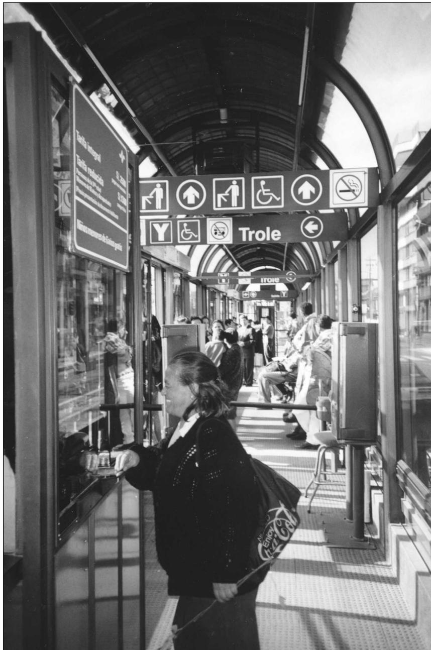
**Figure 4: “Trole” Station Interior with Off-vehicle Fare Collection**
