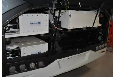
3 LTO battery packs on the vehicle
