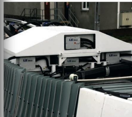
The supercapacitors used for the trolleybuses in Eberswalde are located on the roof.
