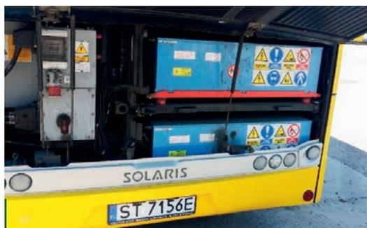
A trolleybus with installed STH600 x84 traction batteries
